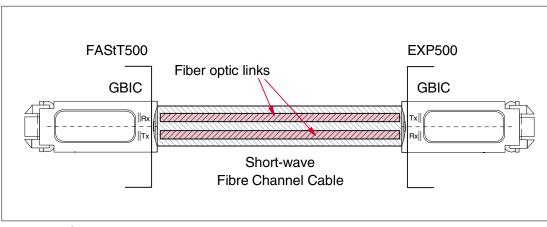
Figure 2-6 Cable diagram
