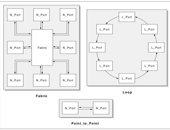
Figure 1-2 Fibre Channel topologies
