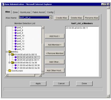
Figure 4-13 Create alias for FAStT500 RAID Controller A
