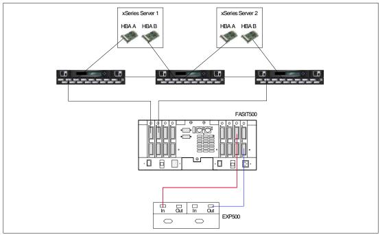
Figure 7-5 Cascaded switch fabric
