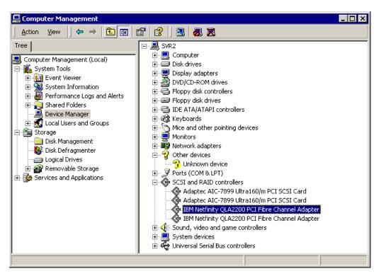
Figure 3-3 Windows automatic device detection
