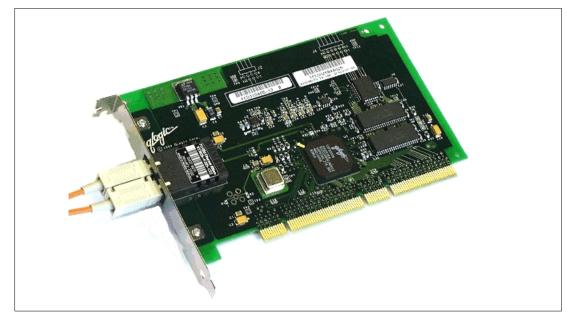
Figure 2-4 FAStT Host Bus Adapter
