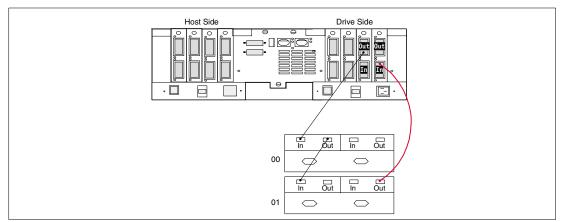
Figure 8-3 Connecting the new EXP500, step 2
